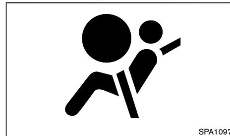
The SRS air bag warning light, displaying
