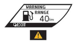
This will appear when the fuel level in the tank is getting low. Refuel as soon as it is convenient, preferably before the fuel gauge reaches the empty (E) position.
