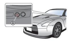
The security indicator light (a) is located in the instrument panel near the windshield. This light operates whenever the ignition switch is in the ACC, OFF or LOCK position. This is normal.
