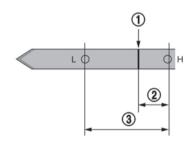
NISSAN recommends to adjust the engine oil level (1) to be 10 mm (0.39 in) (0.5 L) 2 below the H mark on the engine oil dipstick. (3 range is 30 mm
