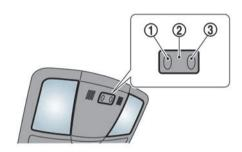
The interior light control switch has three positions: ON ①, DOOR ② and OFF ③.
