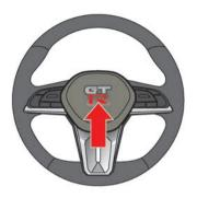
To sound the horn, push the center pad area of the steering wheel.
