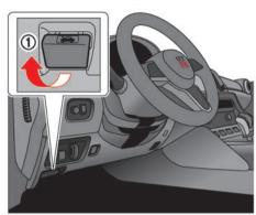
Pull the hood lock release handle 10 located below the instrument panel. The hood will then spring up slightly.
