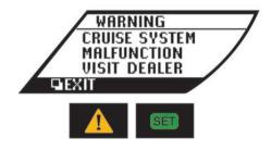
This will appear if the cruise control system is not functioning properly. ( 下至 "Cruise set switch indicator light" page 2-30)
