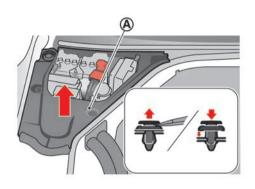
2. Unfasten the 5 clips and remove the cowl top cover (A) by pulling it up.
