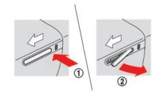
The driver's door will be locked or unlocked using the mechanical key.
