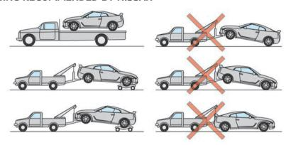
NISSAN recommends that towing dollies be used when towing your vehicle or the vehicle be placed on a flat bed truck as illustrated.
