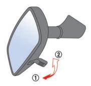
Pull the adjusting lever ① when the glare from the headlights of the vehicle behind vou obstructs your vision at night.
