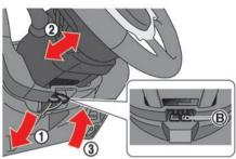
This adjusts the forward/backward position of the steering wheel.
