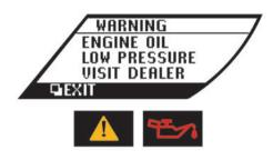
This will appear if the engine oil pressure is low. ( Emgine oil pressure warning light" page 2-26)
