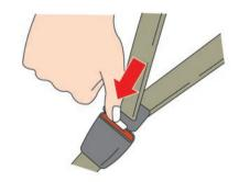
To unfasten the seat belt, push the button on the buckle. The seat belt automatically retracts.
