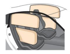
The front side air bags are located in the outside of the seatback of the front seats. The curtain air bags are located in the side roof rails. All of the information, cautions and warnings in this manual apply and must be followed. The side air bags and curtain air bags are designed to inflate in higher severity side collisions, although they may inflate if the forces in another type of collision are similar to those of a higher severity side impact. They are designed to inflate on the side
