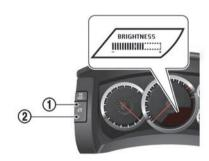
The instrument brightness can be adjusted when the ignition switch is in the ON position. Press the switch to adjust the brightness up ① or down ②. The brightness level is shown on the vehicle information display.
