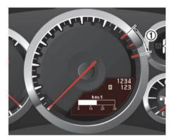
The tachometer indicates the engine speed in revolutions per minute (rpm). Do not rev the engine into the red zone 1).
