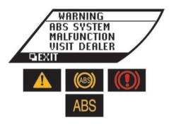
This will appear if the Anti-lock Braking System (ABS) is not functioning properly. (译 "Anti-lock Braking System (ABS) warning light" page 2-24) (译 "Brake warning light" page 2-25)
