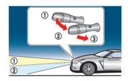
When the headlights are on, push the lever to the front of the vehicle ① to switch to the high beams. The high-beam indicator light illuminates. ( 🎏 "High beam indicator light" page 2-31)
