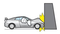
The supplemental front-impact air bag system will deploy in the event of an impact which exceeds a 25 km/h (16 MPH) frontal collision with a solid wall that does not move or deform.
