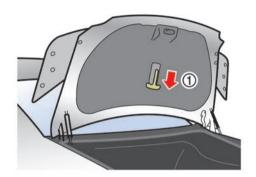
To open the trunk lid from the inside, pull the release handle ① until the lock releases and push up on the trunk lid. The release lever is made of a material that glows in the dark after a brief exposure to ambient light.
