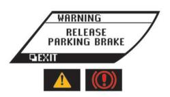
This will appear if the vehicle speed is above 7 km/h (4 MPH) with the parking brake applied. ( Prake warning light" page 2-25) ( 字 "Parking brake reminder chime" page 2-33)
