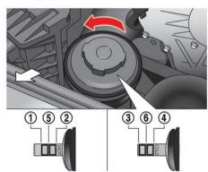
Adjust the power steering fluid level to the R mark (§) on the power steering dipstick when the fluid temperature is hot or  $\ensuremath{\textcircled{6}}$  when the fluid temperature is cold.
