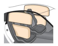
The front side air bags are located in the outside of the seatback of the front seats. The curtain air bags are located in the side roof rails. All of the information, cautions and warnings in this manual apply and must be followed. The side air bags and curtain air bags are designed to inflate in higher severity side collisions, although they may inflate if the forces in another type of collision are similar to
