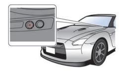
The security indicator light is located on the instrument panel. It indicates the status of the NISSAN Vehicle Immobilizer System.
