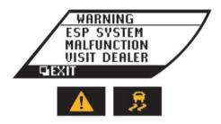
This will appear if the Electronic Stability Program (ESP) system or the hill start assist system is not functioning properly. ( \*\*Technical Electronic Control\*\* (VDC) warning light (except for Europe and India)/Electronic Stability Program (ESP) warning light (for Europe and India)" page 2-30)
