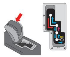
After starting the engine, fully depress the brake pedal and move the shift lever from the **P** position to the **R**. **N**. or  $A \leftrightarrow M$ position. Push the button to shift into the P or R position. All other positions can be selected without pushing the button.
