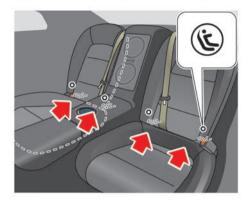
Your vehicle is designed to accommodate a child restraint system on the rear outer seats. Two ISOFIX anchoring points (located between the seat cushion and the seatback) are mounted directly on the body of the vehicle ensuring secure and stable attachment of the child restraint system.
