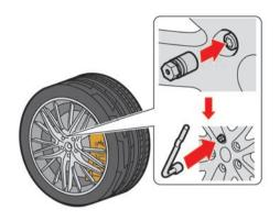
In order to prevent theft, the specially designed wheel lock nut (1) is installed to each wheel. The wheel lock nut cannot be removed with the commonly used tools.
