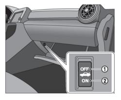
When the switch located inside the glove box is in the OFF position (1), the power to the trunk lid will be canceled and the trunk lid cannot be opened by the trunk lid release switch, the trunk open request switch or the TRUNK button on the Intelligent Key.
