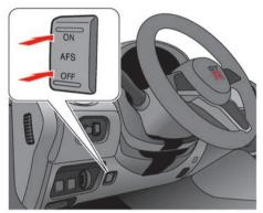
The Adaptive Front lighting System (AFS) will automatically adjust the lighting range of the headlights to improve the driver's view while high-speed driving at night.
