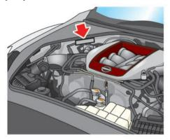
The vehicle identification number is stamped as shown in the engine compartment.
