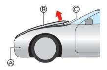
When the sensors (a) (located behind the front bumper) detect an impact above a certain level in frontal collisions, the popup engine hood system will operate and the rear end of the hood (a) is lifted by the lifters (c) instantly.
