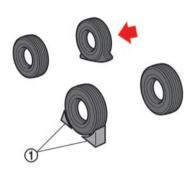
Place suitable blocks (1) at both the front and back of the wheel diagonally opposite the flat tire to prevent the vehicle from moving when it is jacked up.
