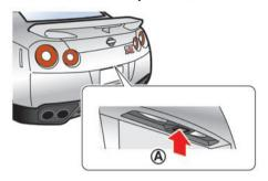
The trunk lid can be opened by pushing the trunk open request switch (A) when the Intelligent Key is within the operating range of the trunk lock/unlock function regardless of the inside lock knob position. ( ) "Intelligent Key system" page 3-
