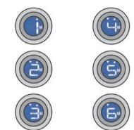
Gear Shift Indicator appears in the transmission position indicator when the driver should shift into a higher or lower gear as indicated by the up or down arrow.
