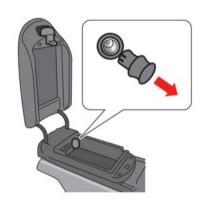
Open the cap to use the outlet. Close the cap after use.
