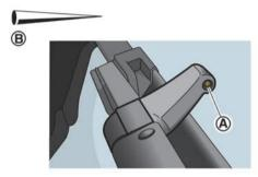
Be careful not to clog the washer nozzle (A. This may cause improper windshield washer operation. If the nozzle is cloqged, remove any objects with a needle or small pin (B). Be careful not to damage the nozzle.
