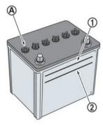
Check the fluid level in each cell (Remove the battery cover if it is necessary). It should be between the UPPER LEVEL (1) and LOWER LEVEL @ lines.
