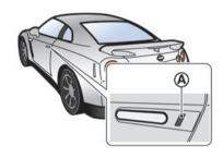
When you carry the Intelligent Key with you, you can lock or unlock all doors by pushing the door handle request switch A within the range of operation.
