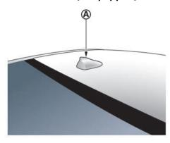
The DAB antenna (A) is located on the rear part of the vehicle roof.
