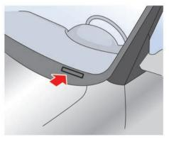
The vehicle identification number plate is attached as shown.
