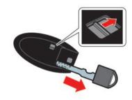
To remove the mechanical key, release the lock knob at the back of the Intelligent Key.
