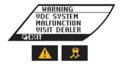
This will appear if the Vehicle Dynamic Control (VDC) system or the hill start assist system is not functioning properly. ( The "Vehicle Dynamic Control (VDC) off indicator light (except for Europe and India)/Electronic Stability Program (ESP) off indicator light (for Europe and India)" page 2-32)
