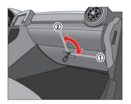
Use the mechanical key to lock ① and unlock ② the glove box. ( >> "Mechanical key" page 3-3)
