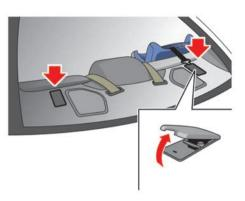
The anchor points are located under the anchorage cover on the rear parcel shelf finisher for the right and left seating positions of the rear seat.
