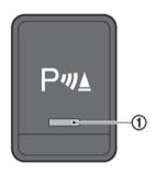
The parking sensor (sonar) system OFF switch on the lower side of the instrument panel allows the driver to turn the parking sensor (sonar) system on and off. To turn the parking sensor (sonar) system on and off, the ignition switch must be in the ON position. The indicator light ① on the switch will turn off when the system is turned off. If the indicator light flashes it may indicate a malfunction in the parking sensor (sonar) system.
