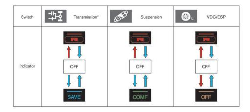
: Push and hold the switch for longer than approximately 1 second
