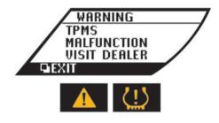
This will appear if the Tire Pressure Monitoring System (TPMS) is not functioning properly. ( ) Low tire pressure warning light" page 2-27)
