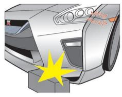
Drive paying careful attention to wheel blocks and curbs. If the front bumper collides with a wheel block etc., the whole bumper may be bent out of shape and parts other than those that were hit (on the bumper side) may be damaged or cracked.
