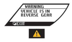
This will appear (and a chime will sound) if the shift lever is in the R position for more than 5 minutes, or when the driver's door is opened while the shift lever is in the R position.
