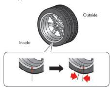
Make sure the tire has not slipped on the wheel causing the assembly to be out of balance. The reference marks on the tire and wheel should be aligned. If the reference marks are not aligned, the tire has slipped on the wheel. Have the wheels/tires rebalanced. Make sure the old reference marks are erased and new reference marks are applied to the wheel and tire. When installing new tires on the wheels, make sure new reference marks are applied to the wheels and tires.
