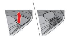
The trunk can be opened with the emergency trunk lid opener located on the floor in front of the passenger's seat.
