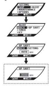
Push the ignition switch to the ON position. Use the ENTER switch 🔲 and toggle the vehicle information display to show the SETTING screen.
