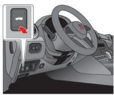
Press the trunk lid release switch to unlock the trunk
