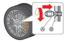
7. Tighten the wheel nuts by hand by turning them clockwise until the tapered part (A) of each nut lightly contacts the seat part ® of the wheel hole.
