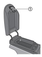
Lift up the lock knob ① to open the lid. To close the center console box, press on the lid until it locks in place.
