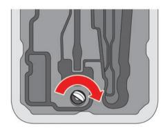
2. Insert the mechanical key into the emergency trunk lid opener and turn it clockwise until it stops.
