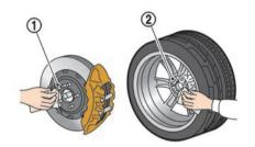
5. Remove the wheel nuts and then remove the wheel.
