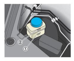
Check the fluid level in the reservoir. If the fluid is below the MIN line ① or the brake warning light comes on, add Genuine NISSAN Brake Fluid R35 Special II fluid up to the MAX line 2). If fluid must be added frequently, the system should be checked by a NISSAN High Performance Center (NHPC).
