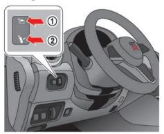
Press the switch down 2 to fold the outside mirrors
