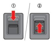
To lock a door individually, push down the inside lock knob to the lock position 1 then close the door.
