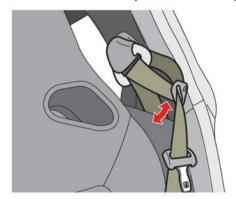
Before fastening the seat belt, adjust the shoulder belt arm to the lock position where the belt fits snugly on the shoulder. The arm can also be folded down to allow rear seat passengers easier access.
