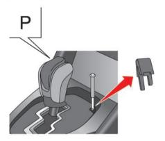
If the battery charge is low or discharged. the shift lever may not be moved from the position even with the brake pedal depressed and the shift lever button pushed.
