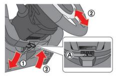
This adjusts up/down the position of the steering wheel.
