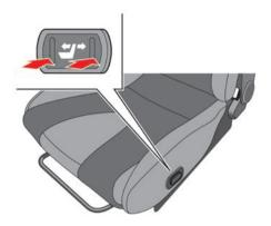
Push each side of the adjustment switch until the desired seatback angle is obtained.
