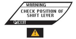
This will appear if the system cannot detect the shift lever position.
