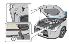
3. Grasp the insulated part of the stay ③ and release it from the hook, then securely insert it into the hood hole 4).
