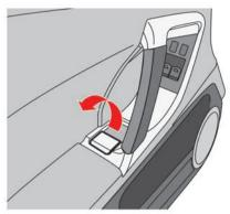
Lift up the inside door handle to open a door from inside the vehicle
