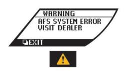
This will appear if the Adaptive Front lighting System (AFS) is not functioning properly. Have the system checked by a NISSAN High Performance Center (NHPC). (译 "Adaptive Front Lighting System (AFS) (except for Mexico)" page 2-58)
