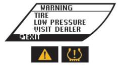
Type B This will appear if the vehicle is being driven with low tire pressure. ( The "Low tire pressure warning light" page 2-27)
