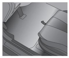
This vehicle includes front floor mat brackets to act as floor mat positioning aid. NISSAN floor mats have been specially designed for your vehicle model. The front floor mats have grommet holes in them. To install, position the mat by placing the floor mat bracket hook through the floor mat grommet hole while centering the mat in the footwell. Periodically check to make certain that the mats are properly positioned.
