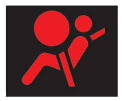
The supplemental air bag warning light, displaying 🖈 in the meter, monitors the circuits for the air bag systems, pretensioner seat belt systems and all related wirings.
