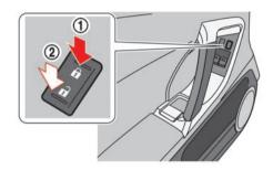
Operating the power door lock switch will lock or unlock all the doors. The switches are located on the driver's and front passenger's door armrests.
