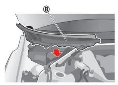
3. Unfasten the 3 clips and remove the cowl top cover ® by pulling it towards the front of the vehicle.
