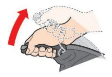
From the released position, pull the parking brake lever slowly and firmly. If the number of clicks is out of the range listed, see a NISSAN High Performance Center (NHPC).
