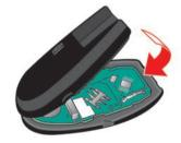
4. Reconnect the upper and lower parts of the Intelligent Key.
