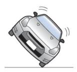
The roof-mounted curtain side-impact and rollover supplemental air bags will deploy in the event of a side impact with a normal passenger vehicle that exceeds at a speed of 25 km/h (16 MPH).
