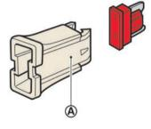
3. Remove the fuse with the fuse puller
