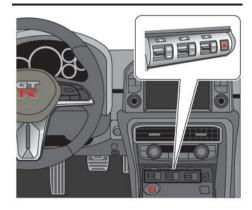
The control of the dual clutch transmission, Bilstein DampTronic® electronically controlled shock absorbers and Vehicle Dvnamic Control (VDC)/Electronic Stability Program (ESP) can be changed to the desired modes by operating the setup switches. Select the desired mode best suited to the driving conditions.
