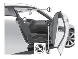
Warning labels about the supplemental front-impact air bag are placed in the vehicle as shown in the illustration.
