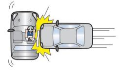
The front seat-mounted side-impact supplemental air bag will deploy in the event of a side impact with a normal passenger vehicle that exceeds at a speed of 25 km/h (16 MPH).
