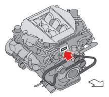
The number is stamped on the engine as shown.
