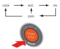
When the Intelligent Key is carried with you and the ignition switch is pushed without depressing the brake pedal, the ignition switch position will change as follows:
