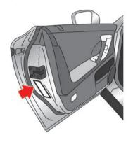
The cold tire pressure is shown on the tire placard label affixed to the door end as illustrated.
