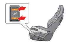
The seat heaters can be used when the ignition switch is in the ON position. The front seats are warmed by the built-in heaters.
