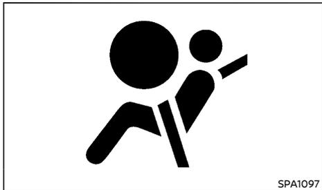
The supplemental air bag warning light, displaying
