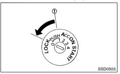
The ignition switch includes a device that helps prevent accidental removal of the key while driving.
