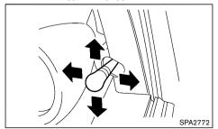
Adjust the mirror angles with the inside lever until the desired position is achieved.
