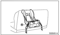
If you must install a rear-facing child restraint system on the rear center seat, follow these steps:
