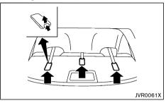
The anchor points are located on the rear parcel shelf for all three seating positions of the rear seat as shown (for Australia).
