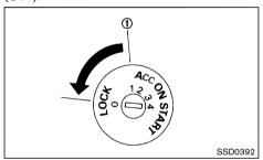
The ignition lock is designed so that the ignition switch cannot be turned to the "LOCK" position until the shift lever is moved to the "P" (Park) position. When moving the ignition switch to the "LOCK" position, to remove the key from the ignition switch, make sure the shift lever is in the "P" (Park) position.
