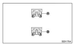
6. If the fuse is open (A), replace it with a new fuse **(B**)
