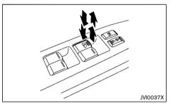
Automatic function is available for the switch that has an /A mark on its surface.
