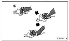
To prevent slack in the lap belt, it is necessary to secure the shoulder belt in place with a locking clip (A). Use the locking clip attached to the child restraint system, or one which is equivalent in dimensions and strength.
