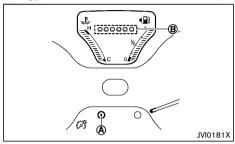
The instrument brightness control (if equipped) operates when the ignition switch is in the "ON" position.
