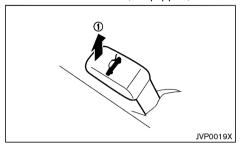
Pull the trunk lid release handle (1) located below the driver's seat until the trunk lid springs up.
