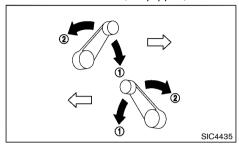
The side windows can be opened ① or closed ② by turning the hand crank on each door.
