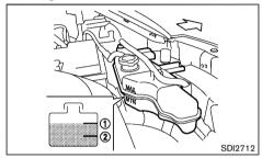
Check the coolant level in the reservoir when the engine is cold. If the coolant level is below the MIN level (2), add coolant up to the MAX level (1).
