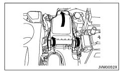
To remove the filter, release the lock pins and pull the unit upward.
