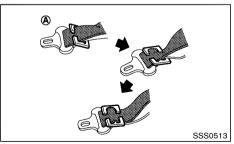
3. To prevent slack in the lap belt, it is necessary to secure the lap belt in place with a locking clip (A) . Use the locking clip attached to the child restraint system, or one which is equivalent in dimensions and strength.
