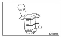
Check the fluid level in the reservoir. If the brake fluid is below the MIN line, the brake warning light will illuminate. Add brake fluid up to the MAX line. (See "Recommended fuel/lubricants and capacities" (P.9-2) for recommended types of brake fluid.)
