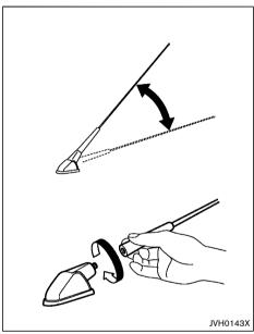
The angle of the antenna can be changed.
