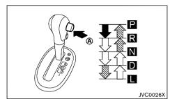
Push the button (A) while depressing the foot brake pedal.
