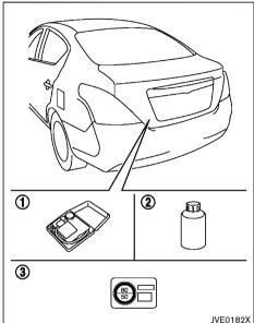
Take out the emergency tire puncture repair kit from the storage area under the trunk. The repair kit consists of the following items:
