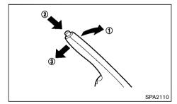
To apply the parking brake, pull the parking brake lever up (1)
