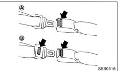
The center seat belt buckle (A) or both the buckle and the tongue (B) are identified by the CENTER mark. The center seat belt tongue can be fastened only into the center seat belt buckle.
