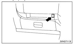
The AUX input jack is located above the glove box. The AUX input jack accepts any standard analog audio input such as from a portable cassette tape/CD player, MP3 player or laptop computer.
