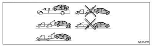
NISSAN recommends that towing dollies be used under the front wheels when towing your vehicle or the vehicle be placed on a flatbed tow truck as illustrated.
