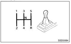
To change gears, or when upshifting or downshifting, fully depress the clutch pedal, shift into the appropriate gear, then slowly and smoothly release the clutch pedal.
