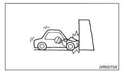
The supplemental front-impact air bag system will deploy in the event of an impact which exceeds a 25 km/h frontal collision with a solid wall that does not move or deform.
