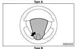
The horn switch operates regardless of the ignition switch position except when the battery is discharged.
