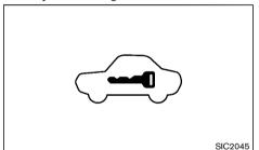
The security indicator light is located in the meter panel.
