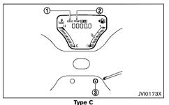
The odometer/twin trip odometer is displayed when the ignition switch is in the "ON" position.
