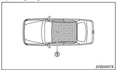
The Intelligent Key can only be used for starting the engine when the Intelligent Key is within the specified operating range (1) as illustrated.
