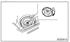
Remove the jack, necessary tools and the spare tire from the storage area.
