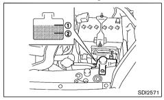
Check the coolant level in the reservoir when the engine is cold. If the coolant level is below the MIN level (2), add coolant up to the MAX level (1). If the reservoir is empty, check the coolant level in the radiator when the engine is cold. If there is insufficient coolant in the radiator, fill the radiator with coolant up to the filler opening and also add it to the reservoir up to the MAX level (1).
