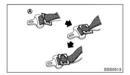
To prevent slack in the lap belt, it is necessary to secure the shoulder belt in place with a locking clip (A). Use the locking clip attached to the child restraint system or one which is equivalent in dimension and strength.
