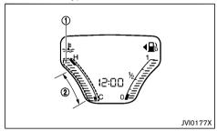
The engine coolant temperature gauge ① indicates the engine coolant temperature.
