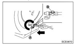
Remove the protective cap (A) of the hose and screw the hose securely onto the tire valve. Make sure that the pressure release valve (B) is securely tightened. Make sure that the air com-
