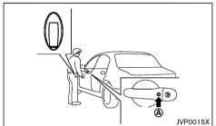
When you carry the Intelligent Key with you, you can lock or unlock all doors by pushing the door handle request switch (driver's or front passenger's) (A) within the range of operation.
