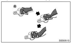
To prevent slack in the lap belt, it is necessary to secure the shoulder belt in place with a locking clip (A). Use the locking clip attached to the child restraint system or one which is equivalent in dimension and strength.
