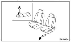
This vehicle includes a front floor mat bracket (A) to act as a floor mat positioning aid. NISSAN floor mats have been specially designed for your vehicle model. The driver's floor mat has a grommet hole incorporated in it.
