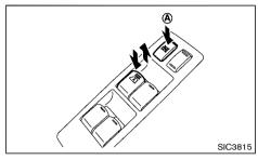
The driver's switch, which is the main switch, can control all windows.
