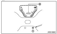
The digital clock ② in the meter displays the time when the ignition switch is in the "ON" position. To adjust the time, perform the following procedure:
