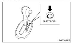
If the battery charge is low or discharged, the shift lever may not be moved from the "P" (Park) position even with the brake pedal depressed and the shift lever button pushed.
