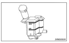
Check the fluid level in the reservoir. If the fluid is below the MIN line, add fluid up to the MAX line. (See "Recommended fuel/lubricants and capacities" (P.9-2) for the recommended types of fluid.)
