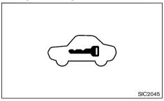
The security indicator light is located on the meter panel. It indicates the status of NATS.
