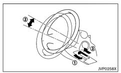
While pushing the lock lever down (1), adjust the steering wheel up or down (2) until the desired position is achieved.
