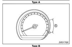
The tachometer indicates the engine speed in revolutions per minute (rpm).
