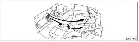
The rear comfort fan improves the comfort level of the rear passengers by sending air-conditioned air from the front seats area to the rear seats.
