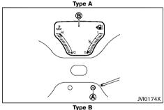
The switch for the trip computer is located on the meter panel  $(\widehat{\mathbf{A}})$ .
