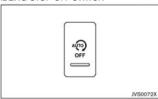
The system can be temporarily deactivated by pressing the Idling Stop System OFF switch. Pressing the switch a second time or restarting the engine by using the ignition switch will reactivate the Idling Stop System.
