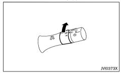
To turn on the rear fog light, turn the fog light switch to the  $\bigcirc$ \$ position with the headlight switch in the EDGE or  $\bigcirc$ Dosition.
