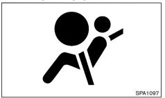
The SRS air bag warning light, displaying 📡 in the instrument panel, monitors the circuits for the air bag systems, pre-tensioner seat belt system and all related wiring.
