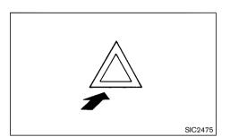
The hazard indicator flasher switch operates with the ignition switch in any position except when the battery is discharged.
