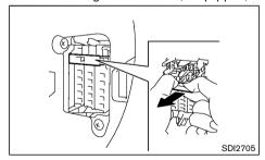
If any electrical equipment does not operate, remove the extended storage fuse switch and check for an open fuse.
