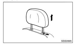
Use the following procedure to remove the adjustable head restraints.
