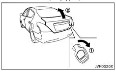
To open the trunk lid, insert the key to the key cylinder and turn the clockwise (1).
