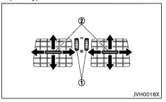
Open/close the ventilators by moving the control (1) in either direction (if equipped).
