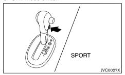
To select the SPORT mode, push the SPORT mode switch with the shift lever in the "D" (Drive) position. The SPORT mode indicator light SPORT in the meter panel illuminates. To turn off the SPORT mode, push the SPORT mode switch again. The SPORT mode indicator light will turn off. When the shift lever is shifted to any position other than "D", the SPORT mode will be automatically turned off.
