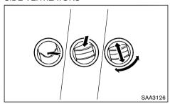
Adjust the air flow direction of the ventilators by opening, closing or rotating.
