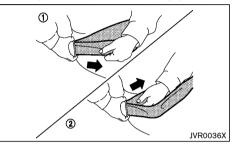
Adjust the seat belt length. To shorten, hold the tongue and pull the upper belt as illustrated (1). To lengthen, hold the tongue and pull the under belt as illustrated (2).
