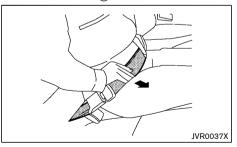
Position the lap belt portion low and snug on the hips as shown.
