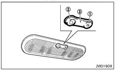
The map light (if equipped) or room light control switch has three positions: ON (1), OFF (2) and center (3).
