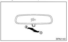
Pull the adjusting lever (1) when the glare from the headlights of the vehicle behind you obstructs your vision at night.
