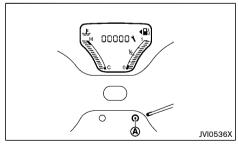
When the ignition switch is placed in the "ON" position, maintenance information (the wrench symbol and distance to change a maintenance item)
